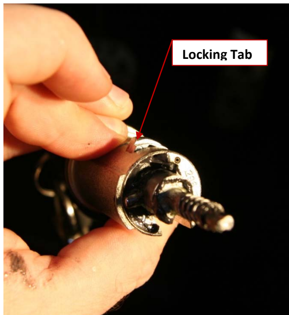
Positioning Key so that Locking Tab can be Depressed
