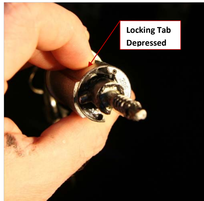
Positioning Key so that Locking Tab can be Depressed
