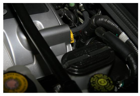
the fuel rail cover. Since one end of this line is fixed to the firewall and the other to the fuel rail, this line is constantly rubbing against the edge of the fuel rail cover as the engine shifts left and right during normal driving. Obviously, more aggressive driving causes even more relative motion and consequently more rubbing.
